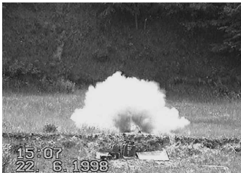
Fig. 5. Propane cloud after tank failure.
